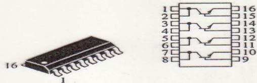
(c) Quad small outline (SO) package for surface-mount technology
